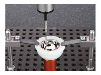
Freeform surface measurement of prosthetic joints can be conducted using a compact, high-accuracy scanning probe with the possibility of performing a three-dimensional error analysis based on the obtained measurement points.
