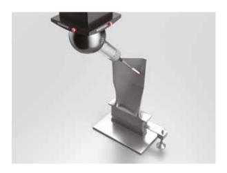
The cross-section of an aircraft engine turbine blade can be measured using a compact, high-accuracy scanning probe that can measure workpieces usually susceptible to large errors, such as castings, quickly and reliably.
