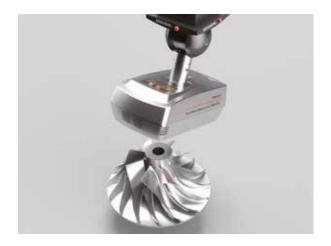
Impellers can be measured using a highly robust non-contact laser probe that reduces multiple reflections. Just as accurate as contact probes, this laser scanner offers high geometric reproducibility.
