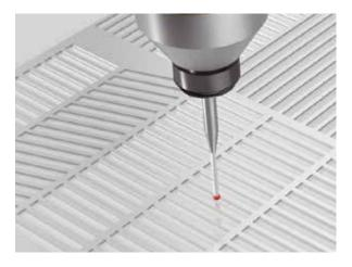
Surface and cross-section measurements of precision molds for separators can be conducted using a low measuring force, high-accuracy scanning probe. Three-dimensional error analysis and cross-sectional form analysis may be performed based on the obtained measurement points.
