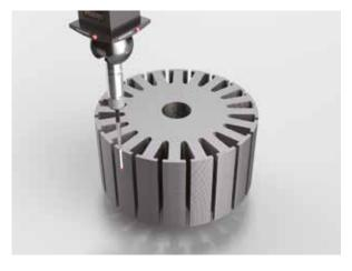
The V Series can measure many sections of laminated motor cores such as straightness or cross-sectional form. It can also conduct measurements of three-dimensional structures, including measurements of side faces and dimensions at arbitrary heights.
